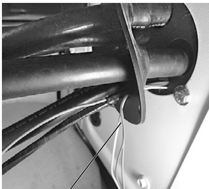
Feed Wiring Harness Through Firewall and Rubber Boot
