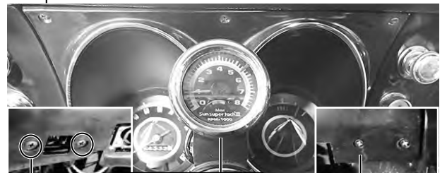
Remove (2) Screws from Bottle Left
